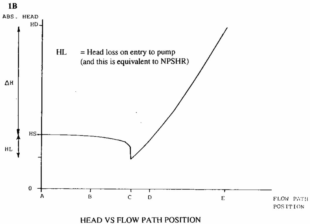
The available NPSH (referred to as NPSHA) is a function of the suction side pumping system and is defined as the absolute pressure head on the liquid surface, plus the static liquid level above the pump centre line (negative for suction lift) minus the friction loss in the piping system leading to the pump minus the vapour pressure head at the pumping temperature. The discharge pumping system has no effect on NPSHA.
