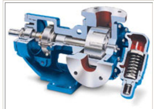
Figure 1. Internal gear pumps are ideal for high-viscosity liquids, but they are damaged when pumping large solids.
