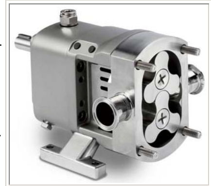
Figure 3. Lobes in lobe pumps do not make contact, because they are driven by external timing gears. This design handles low-viscosity liquids.
